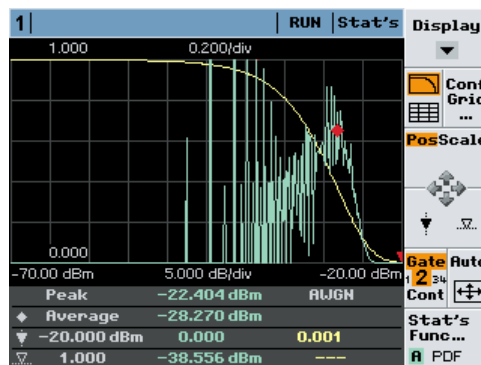
Fig. 4-62: Statistics display mode with two traces (AWGN)
